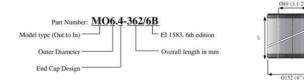
Nominal Length Interchangeable with Flow Rate Model l/min US GPM Velcon mm inch Facet MO6.4-279/6B 160 42 279 11 ACO-61101P FG-O-611 MO6.4-362/6B 56 14 ACO-61401P FG-O-614 212 362 Flat Seal MO6.4-559/6B 365 96 559 22 ACO-62201P FG-O-622 Open Ended MO6.4-727/6B 464 123 727 28 ACO-62901P FG-O-628 MO6.4-842/6B 557 147 842 33 ACO-63301P FG-O-633 MO6.4-1093/6B 756 200 1093 44 ACO-64401P FG-O-644
